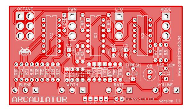
Note that this PCB layout is different than the rullywow.com PCB and uses different BOM's. It also has a few minor changes: added polarity protection, DC filtering and a optional LED trimmer on board.
