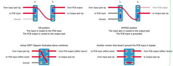
This version is is shown because it's very easy to understand the signalflow here Not recommended by true bypass, but useful in other routing applications
