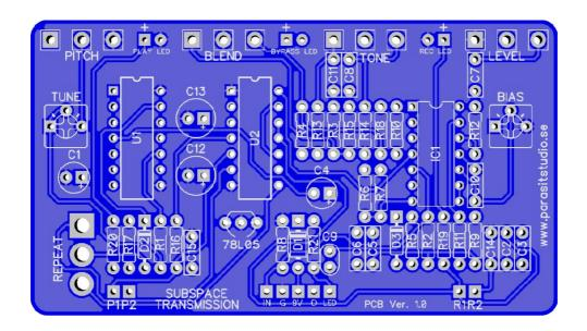
The ISD1820 is a single message chip so you can't use playback and record at the same time to do overdubs. Another drawback is that it always powers down into a powersaving state before starting playback again (even when set to repeat) so fluid repeats that are in cue is hard to achieve. But for a 14-pin DIP chip it's still pretty amazing what it can do!
