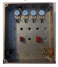
When using a pot cover I usually keep the legs of the pots a bit liften from the hole so that the pot sits flush against the PCB.
