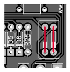
Link the upper and lower pads to have the LFO gate engaged at all times, or just leave it unlinked for a free running LFO.
