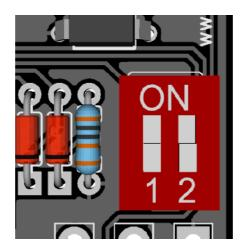
To enable or disable the gate, just turn both dip switches on or off.
