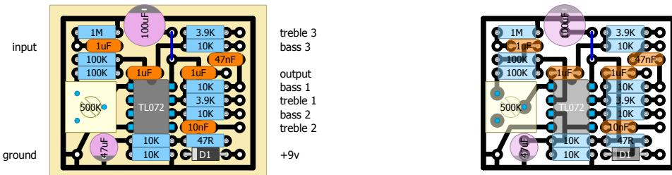
D1: polarity protection diode (1N4001, 1N5817 or 1N4148)
