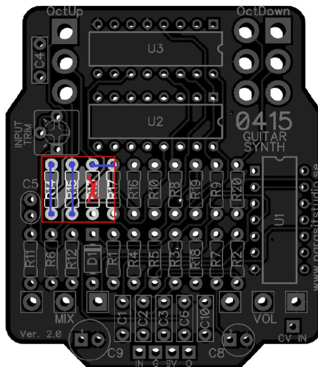
*Even if this shows an unpopulated board, all other components except R13, R14 and R15 should be installed as normal. The blue lines are the 3 links that needs to be soldered in.*
